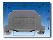
In switchgear and control systems the mounting rails for the terminal blocks are frequently used as protective earth busbars. The PE (protective earth) terminals provide the connection to the mounting rail.
