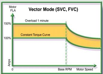
Vector Mode allows operation in either open loop **Sensorless Vector** control or closed loop **Flux Vector** control. Selection between the two is done simply by selecting the Encoder PPR value. Choose a numerical PPR for closed loop operation, or choose "SE" for Sensorless Enhanced open loop operation. In most cases, tuning the drive isn't even necessary when switching between Sensorless and Flux Vector control due to the shared parameter set used for both methods of control.
