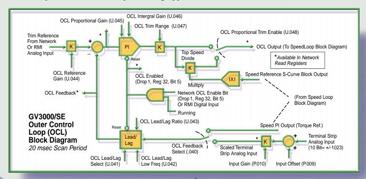
Compensate for inertia build-up in winders.
