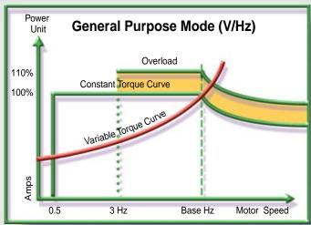
General Purpose Mode **Volts/Hertz** allows classical variable speed control of single or multiple motors from one drive. Operate either squirrel-cage induction or permanent magnet synchronous AC motors in this control mode. It's ideal for applications such as centrifugal fans and pumps, or conveyor applications.
