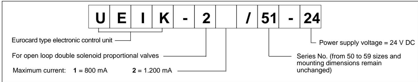
The UEIK-2\* card is an electronic control unit Eurocard type for open loop of double solenoid proportional valves.
