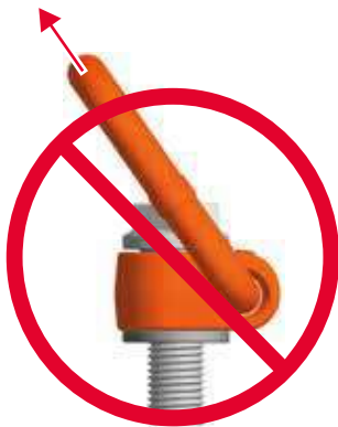
Non-permissible load directions
