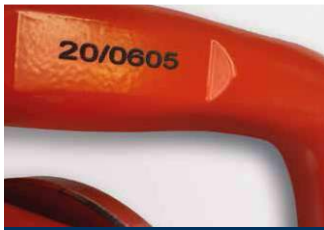
Laser engraved marking of the serial number
