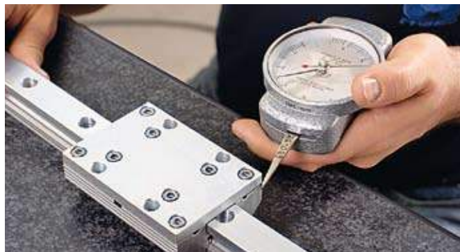
Illustration 2: Measuring Slide Resistance
