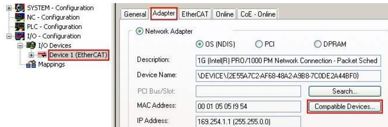
Fig. 109: EtherCAT device properties (TwinCAT 2): click on “Compatible Devices...” of tab “Adapter”
