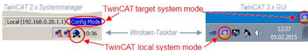
Fig. 132: Differentiation local/target system (left: TwinCAT 2; right: TwinCAT 3)
