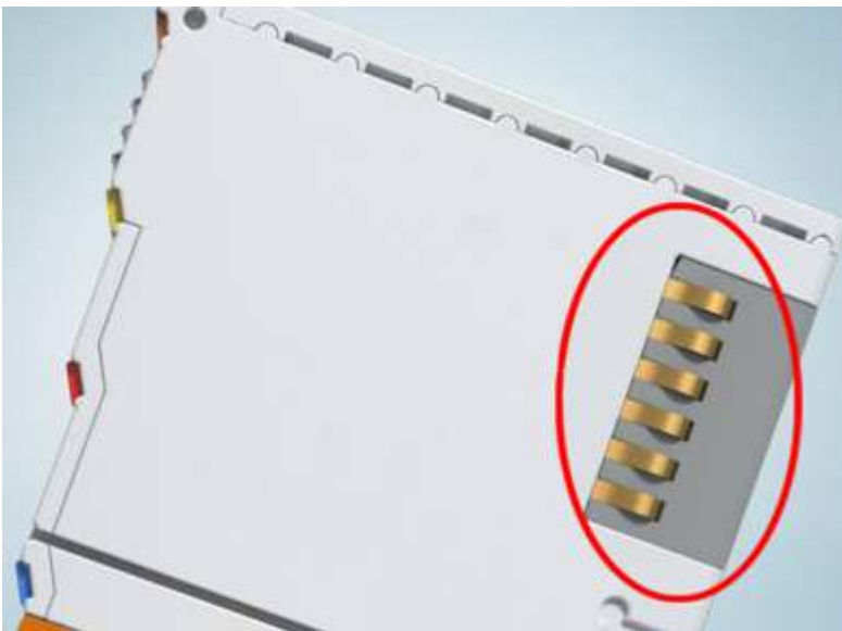
Fig. 51: Spring contacts of the Beckhoff I/O components
