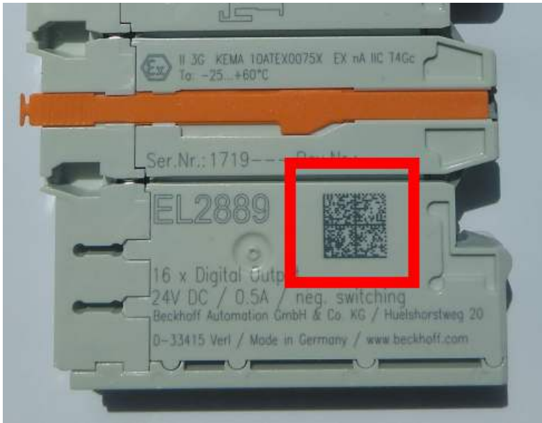
Fig. 2: BIC as data matrix code (DMC, code scheme ECC200)
