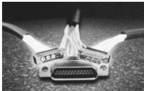
Size Comparison: Above; Nano, Below; Micro-D
