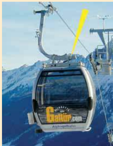
Hydraulic dampers for added convenience when operating cable cars
