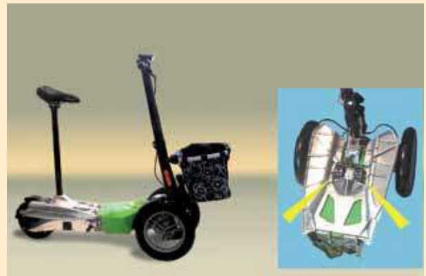
Profile dampers increase the riding comfort of an electric scooter
