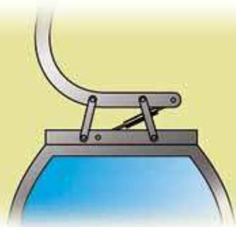
Swinging movements cushioned by hydraulic dampers
