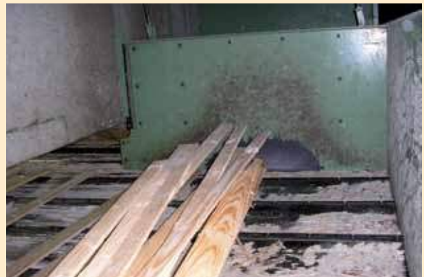
Impact protection for wooden battens
