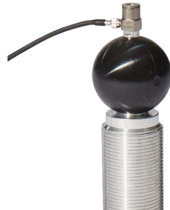
BKS03 (here combined with KS91E Accelerometer )
